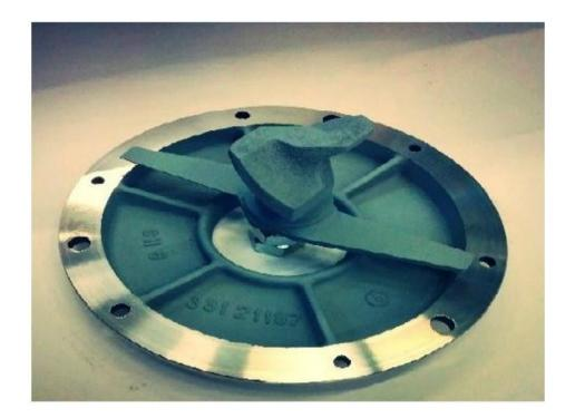
Any application with stringy, fibrous material that needs to be reduced in size is a good chance to use the No clog pump with chopper. Some examples would include pulp and paper, recycling plants, waste water handling and municipal applications.
